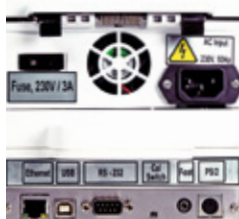
Salida RS232, USB, Ethernet, Foot y PS2
